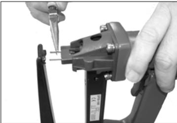
Insert single staple into **Driver Guide(016)**, leaving points protruding.
