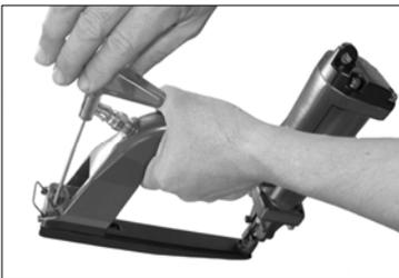
Align **Anvil(029)** with staple points by turning **Screw(506)**.
